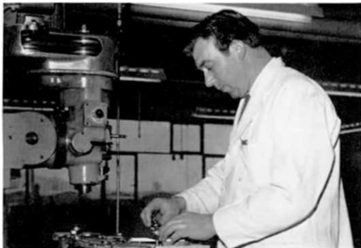
Les Harper machines a casting on a Bridgeport mill.
