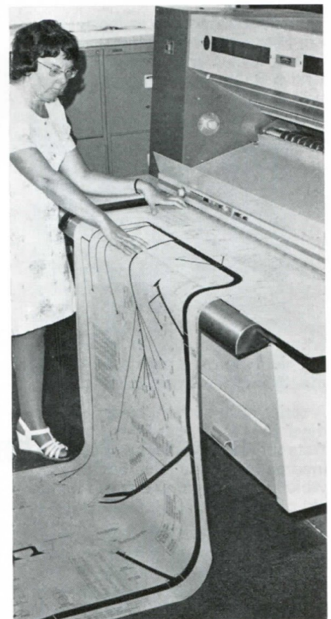
This Ozalid machine produces same size copies of drawings — even when they run to some 6ft in length like this cableform drawing which Jill Trigg is handling.
