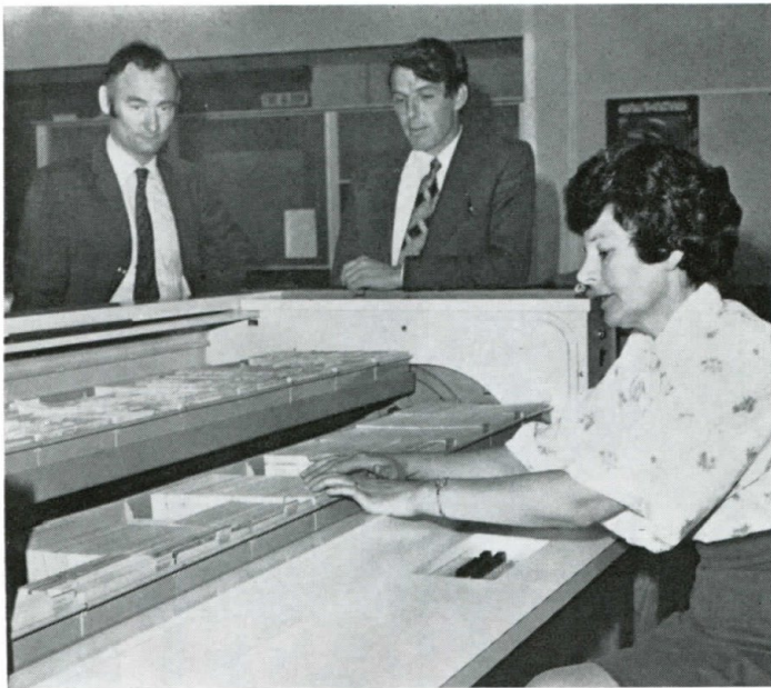
Right: Office Services supervisor Jack Osborne places a drawing on the platen of the camera processor; within half a minute this unit will make a microfilm of a drawing, or part of a drawing, and issue it ready mounted on an aperture card. Using the viewer is Jean McLester.
