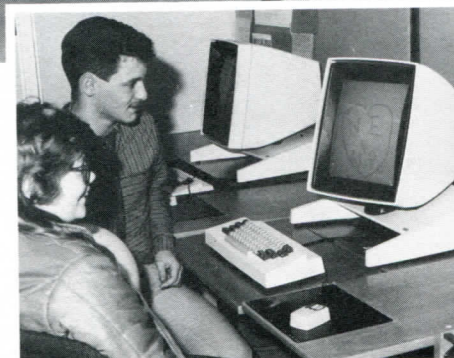
Above: 'Time for new technology' it says on the graphics terminal in MED, as the various facets of the CAD system 'MINT' are explained in colour. Right: Just look what a three-button mouse can do! The grandfathers of our 8000 series, these Alto (c.1973) workstations pioneered the mouse, Ethernet mail and more.
