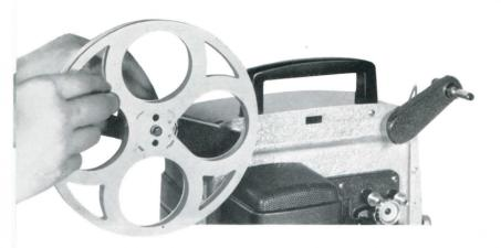
Place the empty reel supplied on the take-up arm spindle and check that this is held securely by the spring clip. Note that the reel will only engage the spindle from one side and must be positioned with the centre slots facing the reel arm.
