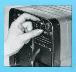
Lay the Moviemaster on its side and locate the Voltage Selector Control and white indicator mark on the base of the projector. Determine the voltage supply to be used. (If in doubt, consult your local electricity authority.) Pull out the Voltage Selector Control and rotate it in either direction until the correct voltage is opposite the white indicator mark, then push in the control until it locates firmly in the socket.
