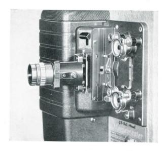
Pull gently on the lens carrier and swing it away from the projector as shown. Flace the reel of film to be shown on the feed arm spindle, and make certain that the reel is securely held in place by the spring clip.
