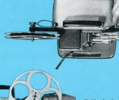
Guide the loose end of film from the take-up reel under the two rollers and insert the end of film in the slot of feed reel. Rotate the feed reel in an anti-clockwise direction to take up the slack.
