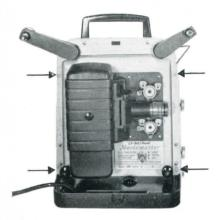
Remove the four screws at front of projector...(Arrowed) and take off the back cover. Disconnect the used belt at the pinched ends and withdraw from the drive pulley.
