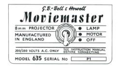
Connect the Moviemaster to the mains supply and place the projector switch to 'Motor', pause momentarily, then switch to 'Lamp'.
