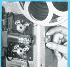
Check for correct threading by turning the threading control clockwise while observing movement of film through the projector. If film loops do not stay in position open the lens carrier and re-position film in the gate and on the sprockets. Check threading before switching on.
