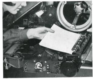
**4.** Fuser Remove any loose sheets of paper in the fuser area. Be careful, the fuser will be quite hot. If a sheet is wrapped around the heat roller, do not try to remove it but send for the Service Engineer.
