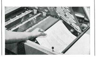
3 As prints were stopped in the copier/duplicator when the mis-feed occurred in the transition module, it is necessary to remove them otherwise it will be impossible to restart the copier/duplicator.
