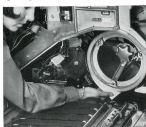
**3b. Register Stop drawer** After having pulled the drawer out as far as it will go, carefully remove any sheets. Check that there are none left behind.
