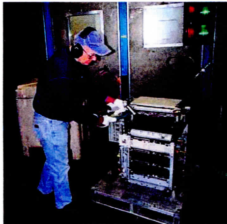
The picture shows Mark Seaborn in ARC's CO 2 cleaning section. All incoming units for asset recycling are cleaned by this process.
