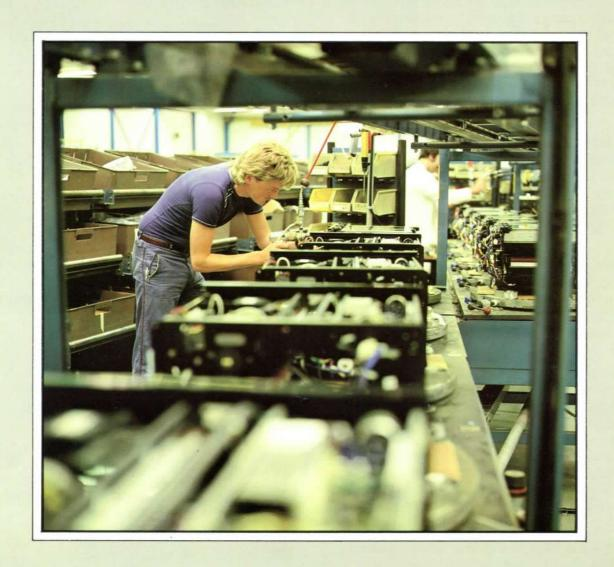
The small copier assembly area at Mitcheldean provides a flexible, cost-effective facility for the production of a range of desk-top models, in volume ranging up to 1000 units per day, dependent on size.
