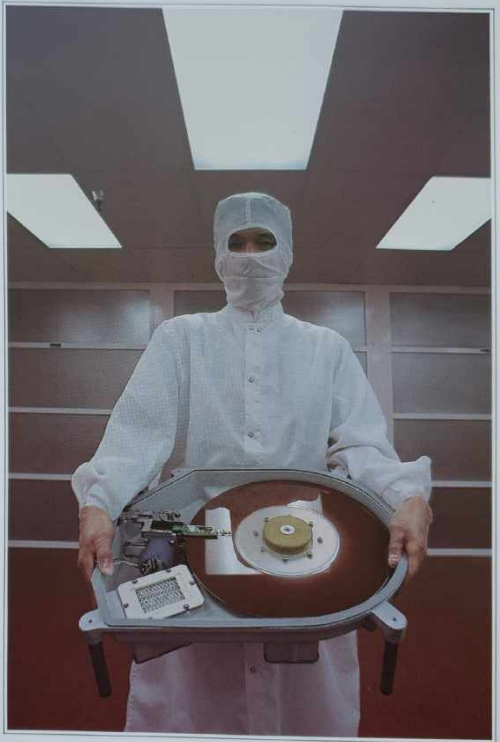
The disc drive assembly room of Century Data Systems Inc., a Xerox company in the USA. The disc drive can store up to three million pages of typed information, any part of which is easily retrievable. The disc drive forms part of advanced office systems.
