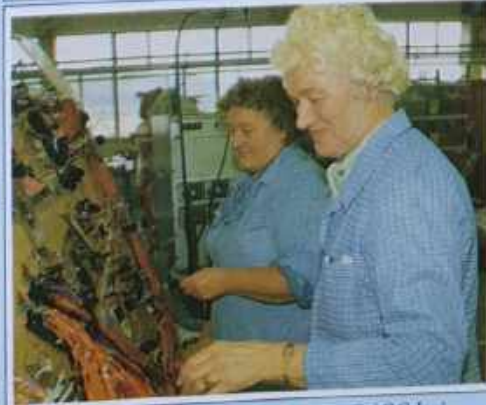
Cable harnesses for the Xerox 9400 being assembled at Mitcheldean by Joan Jones (left) and Eileen Gladwyn.
