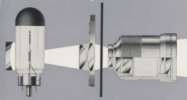
Here's the secret of the Filmosound's exceptionally powerful light output—the straight line optical system which includes an ASPHERIC condenser unit, the precisely located reflector and new Super Proval lens with the remarkably wide aperture of f/1.4.
