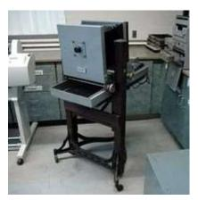
6 - This shows the stand-alone version of the American VR (variable ratio) Camera. It sits on a short chassis, mounted on a heavy-duty tripod stand. There is no copy-board or exposure lamps, so originals needed to be wall mounted and effectively lit, the camera then being rolled up to them. The control panel is on a 'remote' fly-lead, so that operating it wouldn't disturb the camera. The processor sits to the rear.
