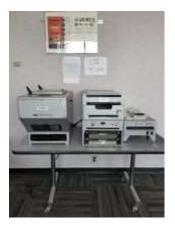
5 - This is exactly the same kit as photo No. 4 but now simply badged as Xerox. The Haloid badging has gone! Note that, in this museum display, the Heat Fuser has been disabled, by removal of its asbestos tray, for health & safety reasons. The useless handle now sits on top.
