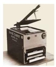
**2 - Haloid XeroX Model A.** The production version of the Ox Box had a much better engineered camera, with a Platen Cover latch and exposure button. The processor is basically the same as the Ox Box, with needle-spray charger. The same fuser was supplied.
